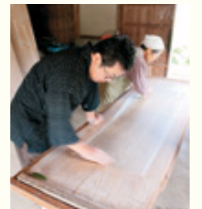
Attaching to drying board
